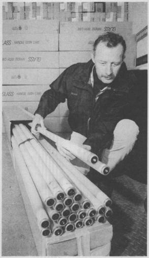
DAVID SZKLARZ of Waste Operations Dept. 7577 examines fluorescent lamps being stored in preparation for shipment to a recycling facility. The glass tubes, aluminum ends, and mercury will be recovered and reused.
